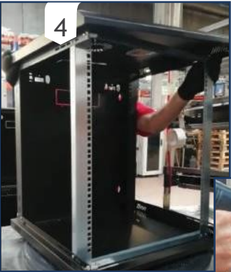
Rear Panel and Top Assembly
