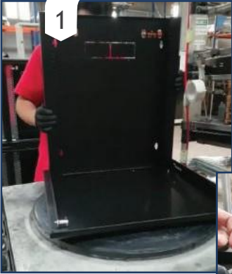
Base and Rear Panel Assembly
